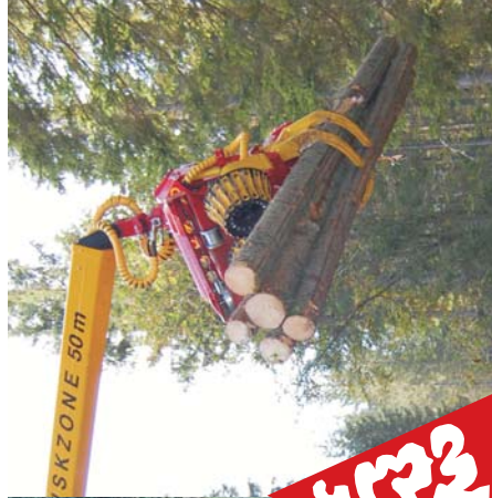
The upwards foldable feeding unit, allows a fully operational loading grapple with endless rotation
